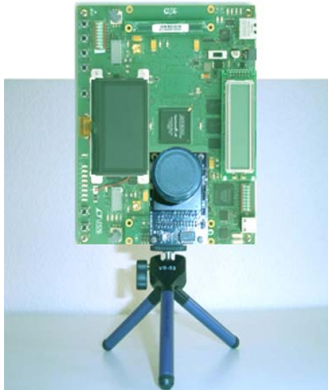
Figure 5. A Complete HD Surveillance System based on an Altera Cyclone III Development Platform
